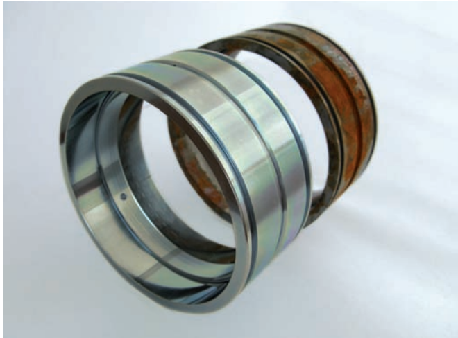
Coated (front) shows no noticeable traces of corrosion after salt spray test. The uncoated control part (back) is rusty.
