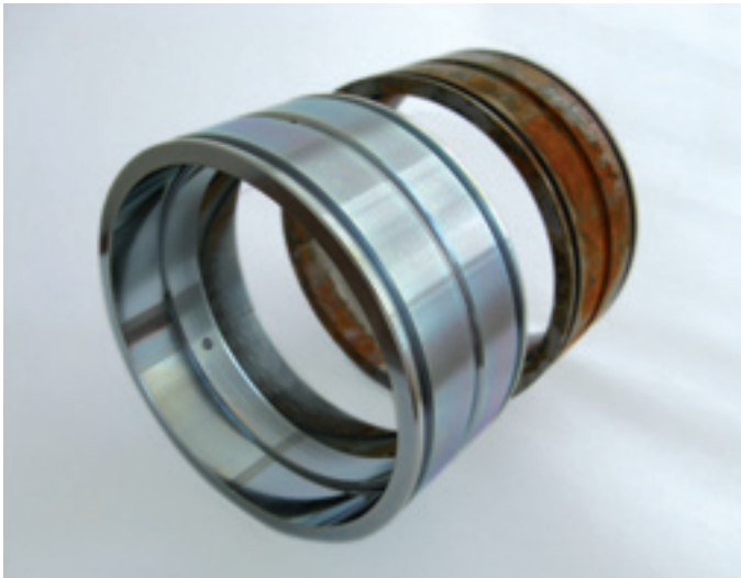
Coated (front) shows no noticeable traces of corrosion after hours of salt spray test. The uncoated control part (back) is rusty.
