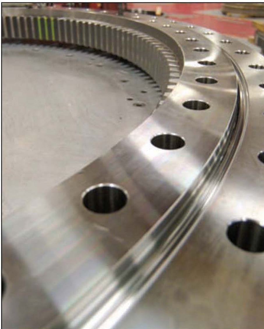
An up-close-and-personal view of a nearly completed wind turbine bearing at Rotek. (Photos courtesy of Rotek.)
