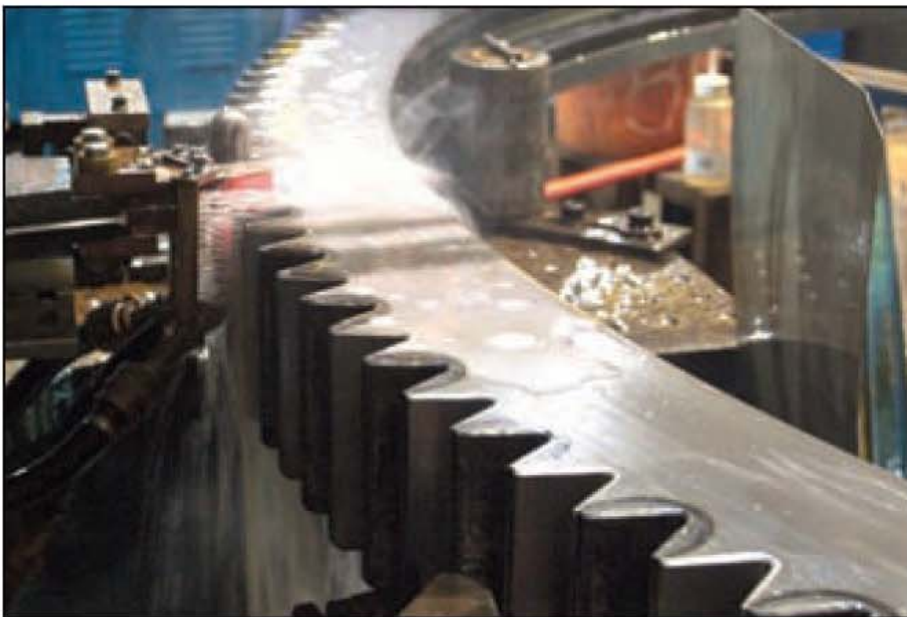
Like most wind turbine bearing manufacturers, Rotek is a one-stop shop. That includes gear hardening, as seen here.
